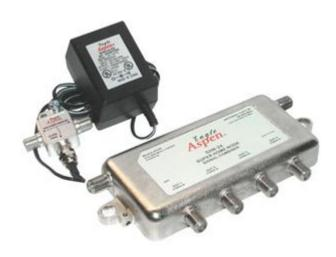
These devices are splitters with built-in amplifiers. Some units contain a potentiometer that increases or decreases the amount of signal from the booster as needed. This is used to counteract the effects associated with multiple splitters and long cable runs. Like taps, diplexers, and non-amplified splitters, these amplified splitters resemble a small metal box with one input leg and two or more output legs.
