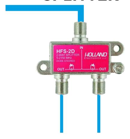
As their name suggests, splitters evenly separate signal among the output legs. These units are often used to go straight to receivers or tuners. (Taps are primarily used to go to infrastructure devices such as multiswitches and modulators.) The amount of loss that's significant depends upon the incoming signal level. Like taps, splitters also experience a port loss of at least 3dB or roughly half the signal. Splitters typically experience a certain amount of insertion loss on each output legs:
